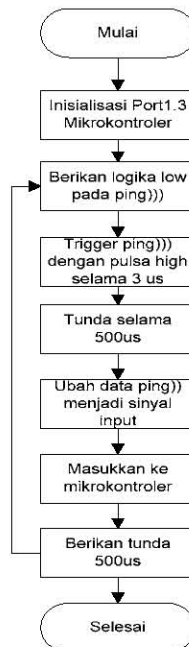
Gambar 10. Diagram Subrutin Sensor
