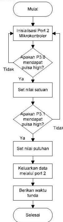
Gambar 11. Diagram Subrutin Display Seven Segment
