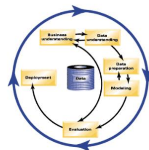
Sumber : Larose, Daniel T, Data Mining Methods and Models Gambar 1.2 Proses CRISP-DM
