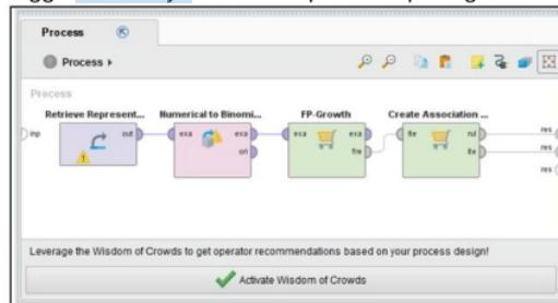
Gambar 3. Susunan Operator Algoritma Apriori
